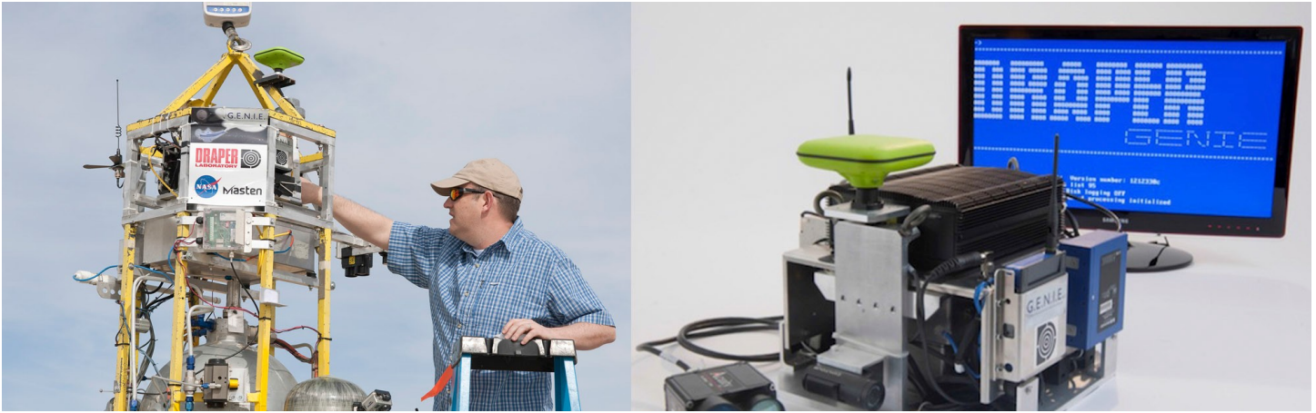
Figure 3 The GENIE autonomous guidance, navigation and control system is shown on the right and is shown mounted on the Masten Space Systems vehicle, Xombie, on the left.
