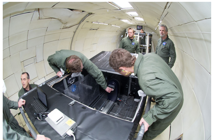
Figure 2 Fine Water Mist Portable Fire Extinguisher developed by ADA Technologies is being prepared for flight testing onboard the Boeing 727 aircraft.
