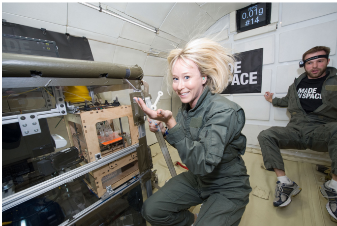
Figure 1 3D printing technology being tested onboard the Boeing 727 aircraft by Made in Space Inc. A nylon wrench that has just been printed in microgravity is floating above the researcher’s hand.
